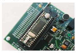
Using the VR Stamp<sup>™</sup> Toolkit, application programs can be downloaded into the VR Stamp<sup>™</sup>. VR Stamp<sup>™</sup> can then be removed from the VR Stamp Programmer<sup>™</sup> and plugged directly into the final product. In-circuit reprogramming is also supported.
