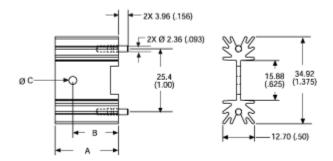
A Dim **38.1 (1.50)**B Dim **18.29 (.720)**C Dim **3.18 (.125)**
