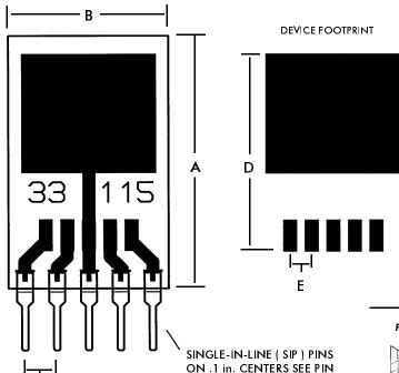
PINS ON .1 in CENTERS PROVIDE COMPATIBILITY WITH BREADBOARDS AND SOCKETS.
