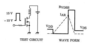
$$\begin{aligned} &R_G = 25~\Omega \\ &V_{DD} = 50~V,~L = 1.74~mH \end{aligned} \qquad E_{AS} = \frac{1}{2} \cdot L \cdot I^2 \cdot \left( \frac{BVDSS}{BVDSS - V_{DD}} \right) \end{aligned}$$
