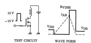
$$\begin{aligned} &RG = 25~\Omega \\ &V_{DD} = 90~V,~L = 1.79~mH \end{aligned} \qquad E_{AS} = \frac{1}{2} \cdot L \cdot I^2 \cdot \left( \frac{B_{VDSS}}{B_{VDSS} - V_{DD}} \right)$$
