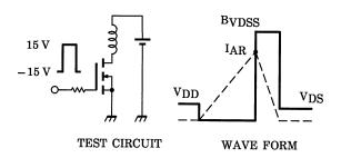
$$\begin{aligned} &R_G = 25~\Omega \\ &V_{DD} = 50~V,~L = 1.74~mH \end{aligned} \qquad E_{AS} = \frac{1}{2} \cdot L \cdot I^2 \cdot \left( \frac{BV_{DSS}}{BV_{DSS} - V_{DD}} \right)$$
