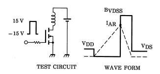
$$\begin{aligned} R_G &= 25~\Omega \\ V_{DD} &= 25~V,~L = 10~mH \end{aligned} \qquad E_{AS} &= \frac{1}{2} \cdot L \cdot I^2 \cdot \left( \frac{B_{VDSS}}{B_{VDSS} - V_{DD}} \right) \end{aligned}$$
