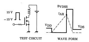
$$\begin{aligned} R_G &= 25~\Omega \\ V_{DD} &= 90~V,~L = 24.9~mH \end{aligned} \qquad E_{AS} &= \frac{1}{2} \cdot L \cdot I^2 \cdot \left( \frac{Bv_{DSS}}{Bv_{DSS} - V_{DD}} \right) \end{aligned}$$
