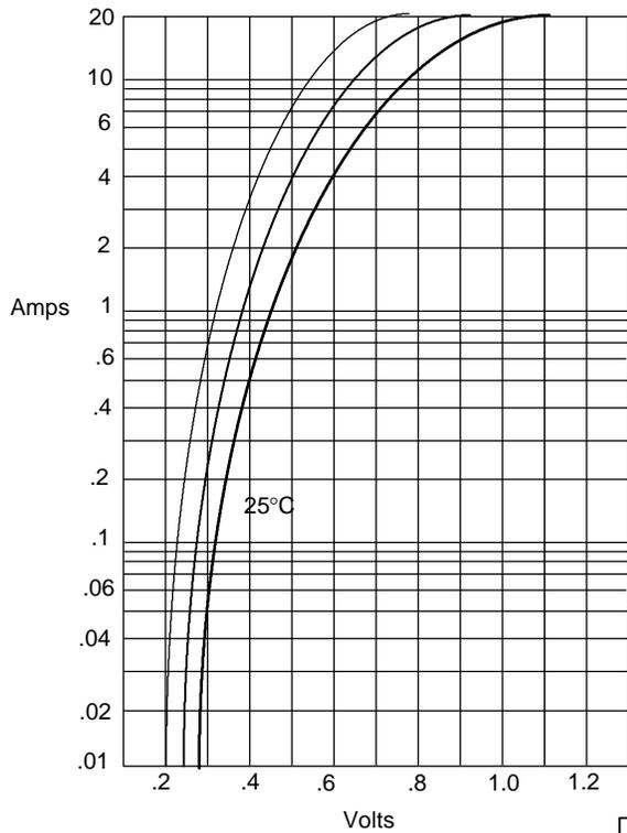
Instantaneous Forward Current - Amperes *versus*
