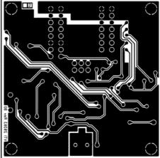
Figure 17. CMA3000 DEMO KIT USB interface board PWB layout.
