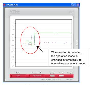
Figure 6. Scroll display with detected motion.
