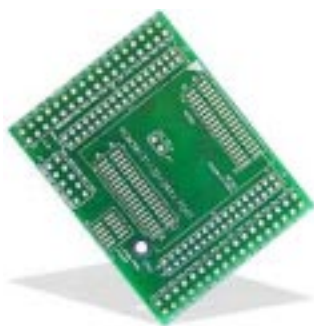
Adapter Board for Rabbit 3000 Based RabbitCore Modules
