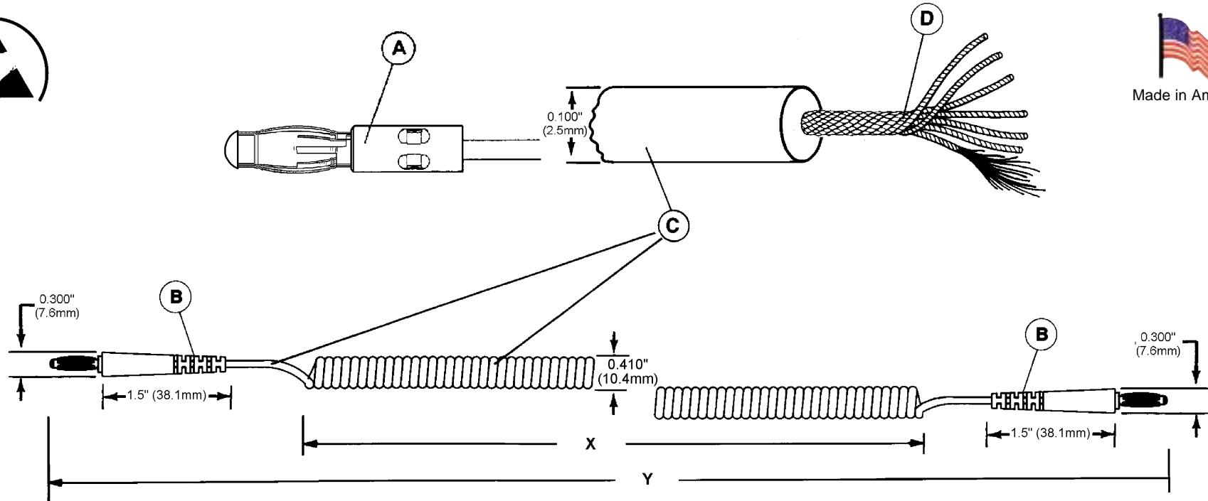
Banana-Banana Coil Cord allows cart users to ground carts to common grounding point on a bench.
