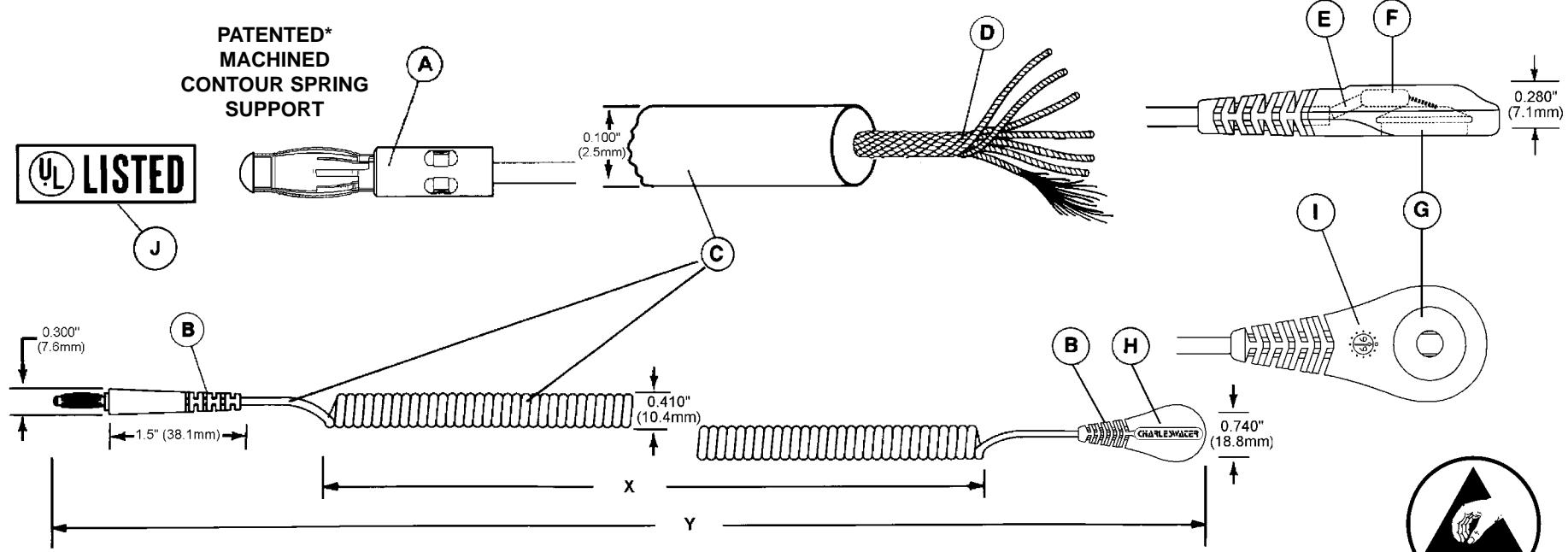
A. Patented\* barrel type banana plug with **machined contour spring support**. Crimped uniformly from 4 sides for maximum strength. Fits industry standard banana jack  $\geq .157"$ . Will maintain greater than 1 pound disengagement force over the life of the cord.
