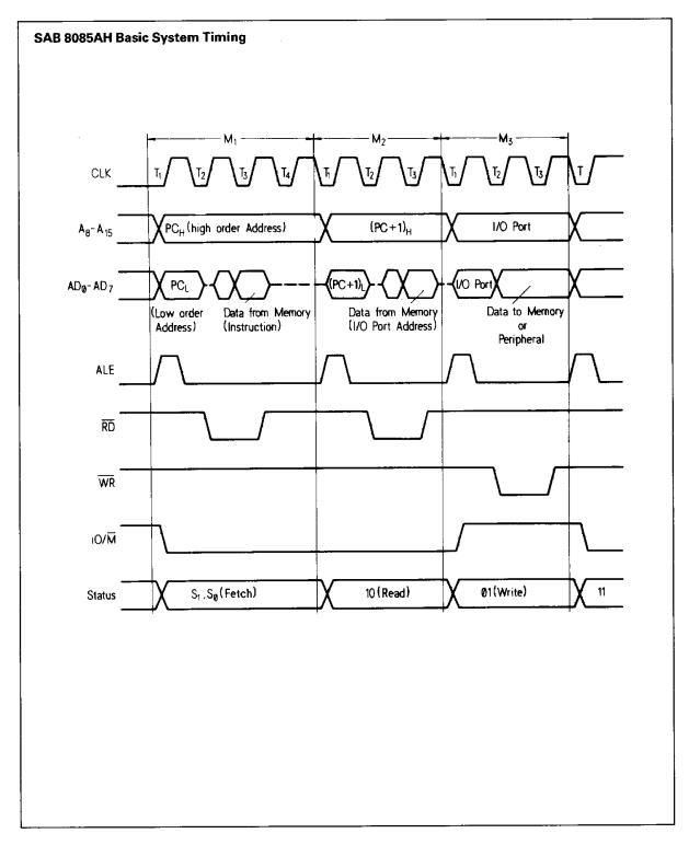
There are seven possible types of machine cycles. Which of these seven takes place is defined by the status of the three status lines ( $IO/\overline{M}$ ,  $S_1$ ,  $S_0$ ) and the three control signals ( $\overline{RD}$ ,  $\overline{WR}$ , and  $\overline{INTA}$ ); (see following table). The status lines can be used as advanced controls (for device selection, for example),
