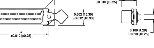
050 GENDER 2 = FEMALE **TERMINATION** 0 = SOLDER CUP RoHS COMPLIANT L = LOW TEMP. PROCESS SHELL PLATING 3 = NICKEL HARDWARE -00 = NO HARDWARE PLATING -1 = GOLD FLASH
