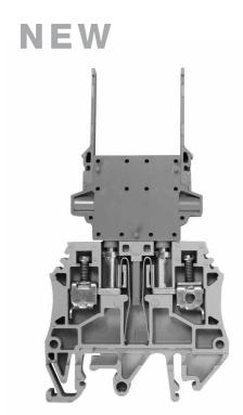
Disconnect test terminals are put to use in all kinds of applications where it becomes necessary to tap into the electrical circuits for test and control purposes. In order to perform the measuring procedure as quickly as possible, the test adapter must be quick and easy to connect. Together with the corresponding test adapters, the new WTL 4/2 STB facilitates disconnecting the circuit by opening the busbar and connecting to the test sockets in a single movement.
