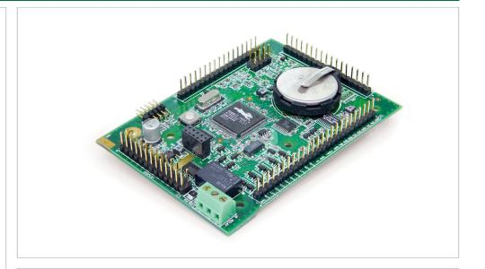
The LP3500 is a low-power single-board computer designed to operate reliably in any place it is deployed, especially where power is limited, such as in portable, hand-held, battery-powered, remote monitoring systems. The LP3500 features built-in analog and digital I/O, while consuming less than 20 mA when fully operational and less than 100  $\mu$ A in power-save mode.
