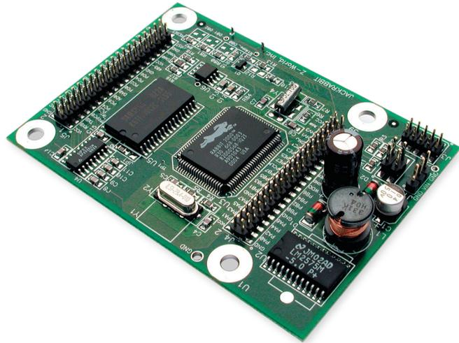
The BL1800 Jackrabbit is a small, easy-to-use, single-board computer that offers reliable hardware for embedded applications.
