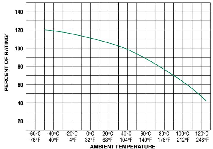
• Ambient temperature effects are in addition to the normal derating.
