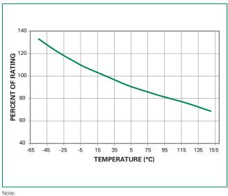
1. Derating depicted in this curve is in addition to the standard derating of 20% for continuous operation.
