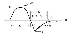
Figure 15. Diode Reverse Recovery Waveform
