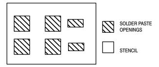
Figure 17. Typical Stencil for DPAK and D<sup>2</sup>PAK Packages
