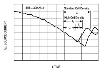
Figure 11. Reverse Recovery Time (t<sub>rr</sub>)
