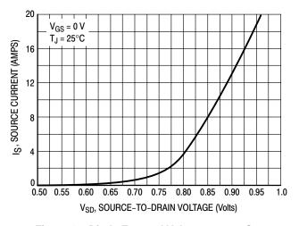
Figure 10. Diode Forward Voltage versus Current
