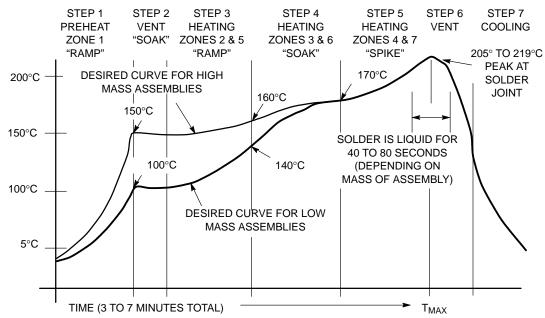
Figure 18. Typical Solder Heating Profile
