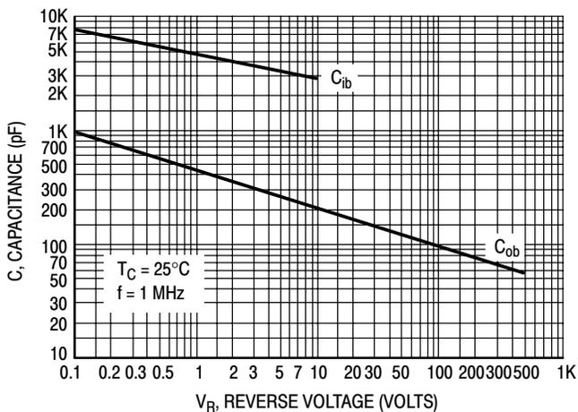
Figure 5. Typical Capacitance
