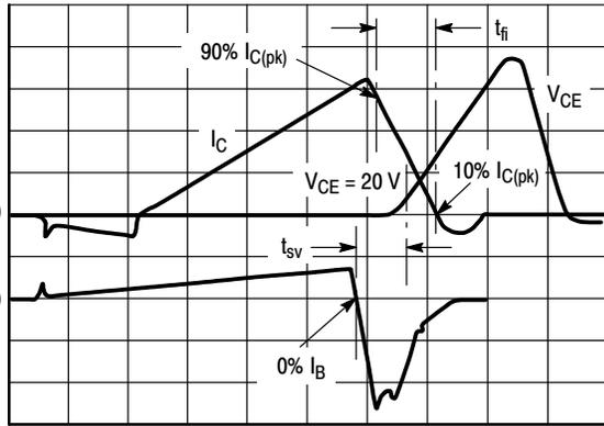
Figure 13. Deflection Simulator Switching Waveforms From Circuit in Figure 15
