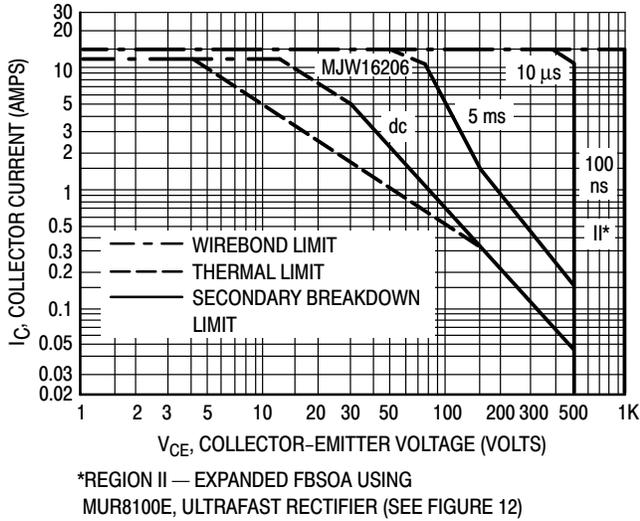
Figure 7. Maximum Forward Biased Safe Operating Area
