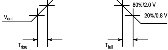
Figure 14. Waveforms: Rise and Fall Times
