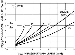
Figure 4. Typical Power Dissipation
