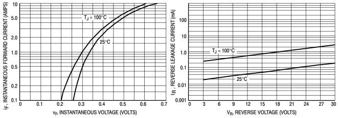
Figure 1. Typical Forward Voltage
