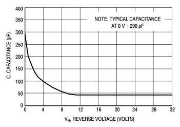
Figure 5. Typical Capacitance
