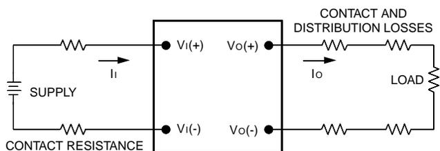
Note: All measurements are taken at the module terminals. When socketing, place Kelvin connections at module terminals to avoid measurement errors due to socket contact resistance.
