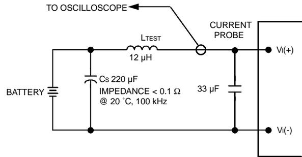
Note: Input reflected-ripple current is measured with a simulated source impedance of 12  $\mu$ H. Capacitor Cs offsets possible battery impedance. Current is measured at the input of the module.
