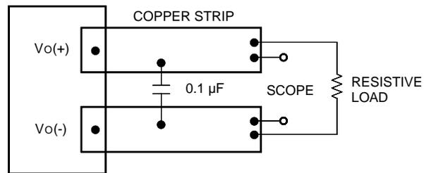
Note: Use a 0.1  $\mu$ F ceramic capacitor. Scope measurement should be made using a BNC socket. Position the load between 50 mm and 75 mm (2 in. and 3 in.) from the module.
