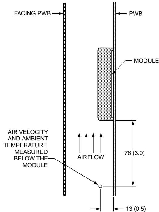
Note: Dimensions are in millimeters and (inches).
