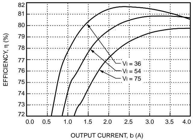
Figure 5. LW020A Typical Converter Efficiency vs. Output Current
