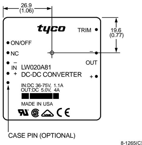
Note: Dimensions are in millimeters and (inches). Pin locations are for reference only.
