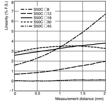
Material of Sensing Object vs. Linearity (with Linearity Adjusted for Each Sensing Object)
