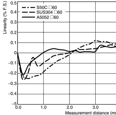
Material of Sensing Object vs. Linearity (with Linearity Adjusted for Standard Sensing Object and Iron)
