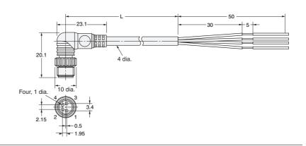
● S8 Snap-in Connectors with Vibration-proof Robot Cable
