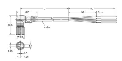
● S8 Snap-in Connectors with Vibration-proof Robot Cable
