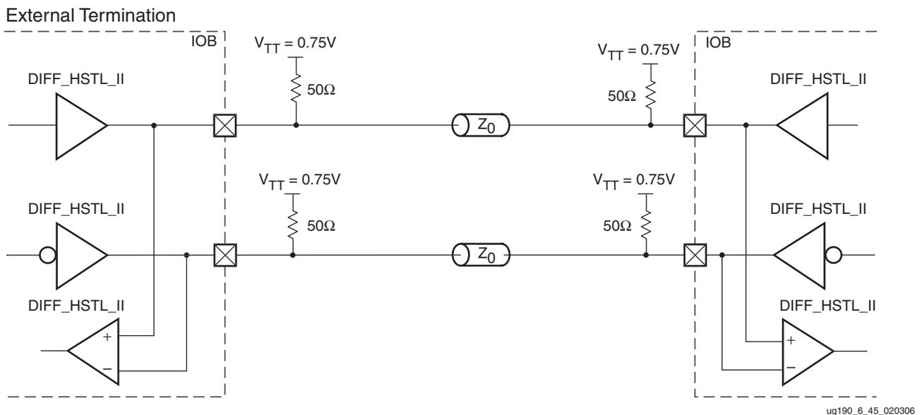
Figure 6-47: Differential HSTL (1.5V) Class II Bidirectional Termination
