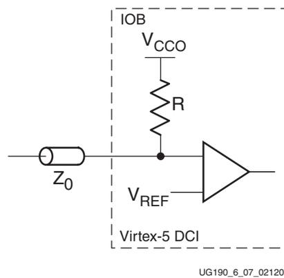
Figure 6-9: Input Termination Using DCI Single Termination
