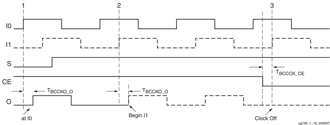
Figure 1-16: BUFGMUX\_VIRTEX4 with a CE Timing Diagram
