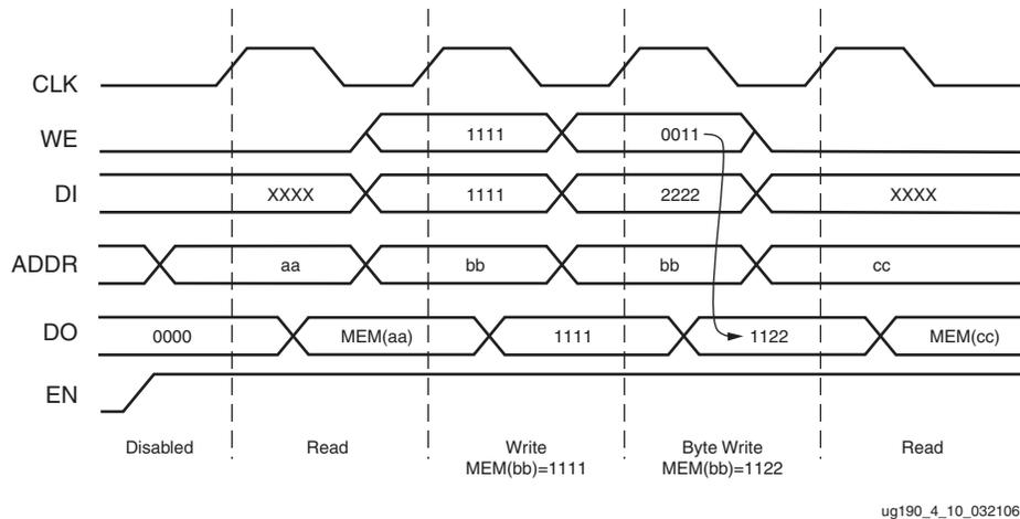
Figure 4-8: Byte-wide Write Operation Waveforms (x36 WRITE\_FIRST)
