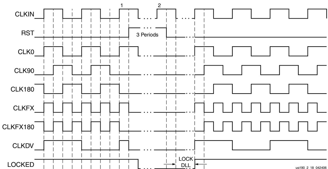
Figure 2-17: RESET/LOCK Example
