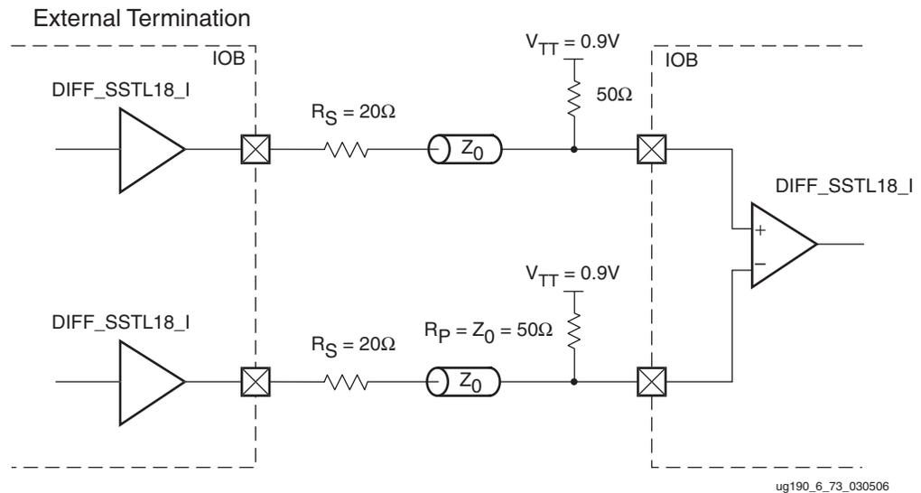
Figure 6-78: Differential SSTL (1.8V) Class I Unidirectional Termination
