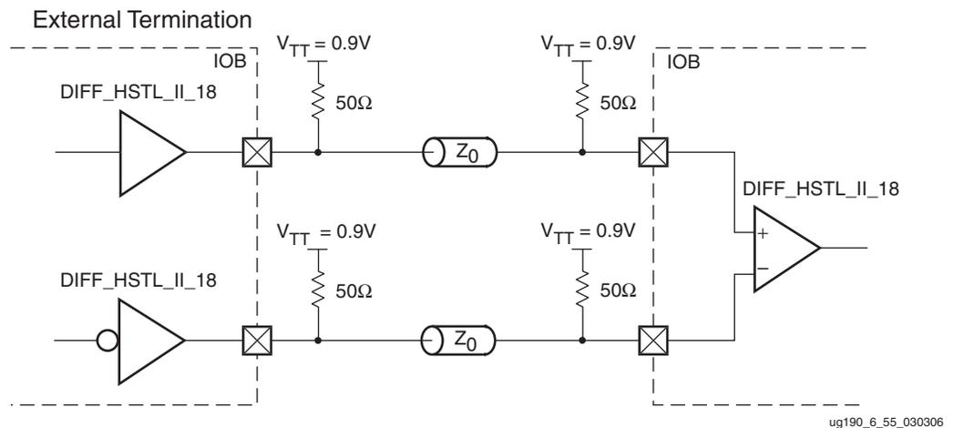
Figure 6-58: Differential HSTL (1.8V) Class II Unidirectional Termination
