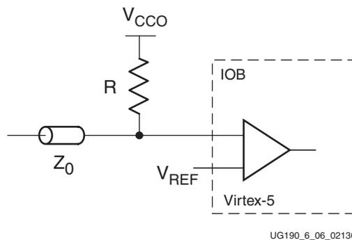
Figure 6-8: **Input Termination to  $V_{CC0}$  without DCI**
