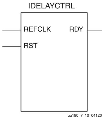
Figure 7-15: IDELAYCTRL Primitive
