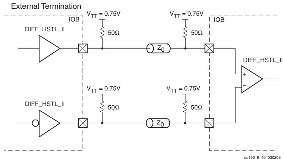
Figure 6-45: Differential HSTL (1.5V) Class II Unidirectional Termination
