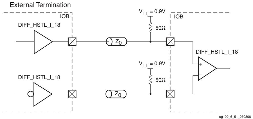
Figure 6-54: Differential HSTL (1.8V) Class I Unidirectional Termination
