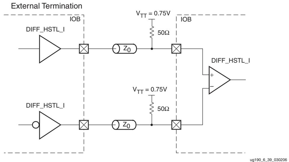
Figure 6-41: Differential HSTL (1.5V) Class I Unidirectional Termination
