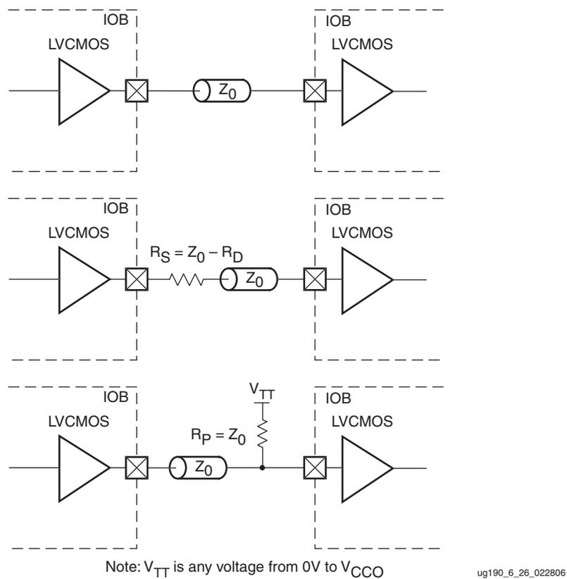
Figure 6-29: LVCMOS Unidirectional Termination
