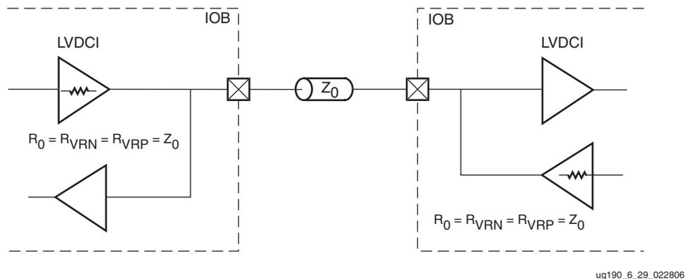
Figure 6-32: Controlled Impedance Driver with Bidirectional Termination
