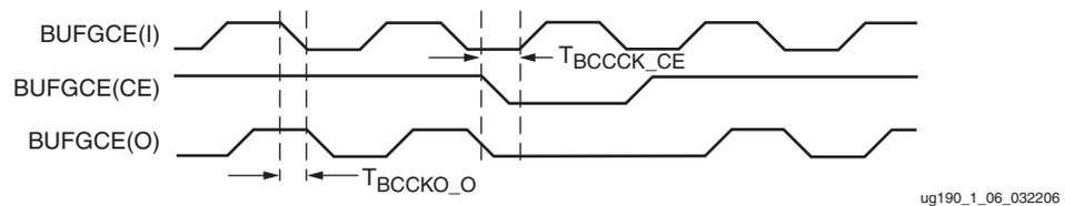
Figure 1-6: **BUFGE Timing Diagram**
