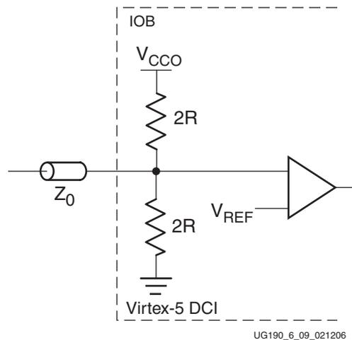
Figure 6-11: Input Termination to  $V_{CC0}/2$  Using DCI Split Termination
