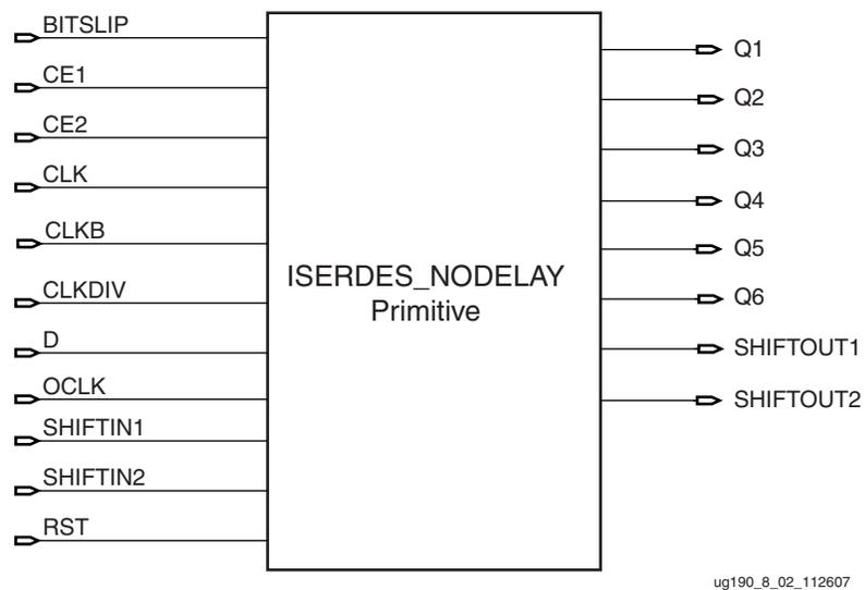
Figure 8-2: ISERDES\_NODELAY Primitive
