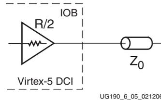
Figure 6-7: **Controlled Impedance Driver with Half Impedance**
