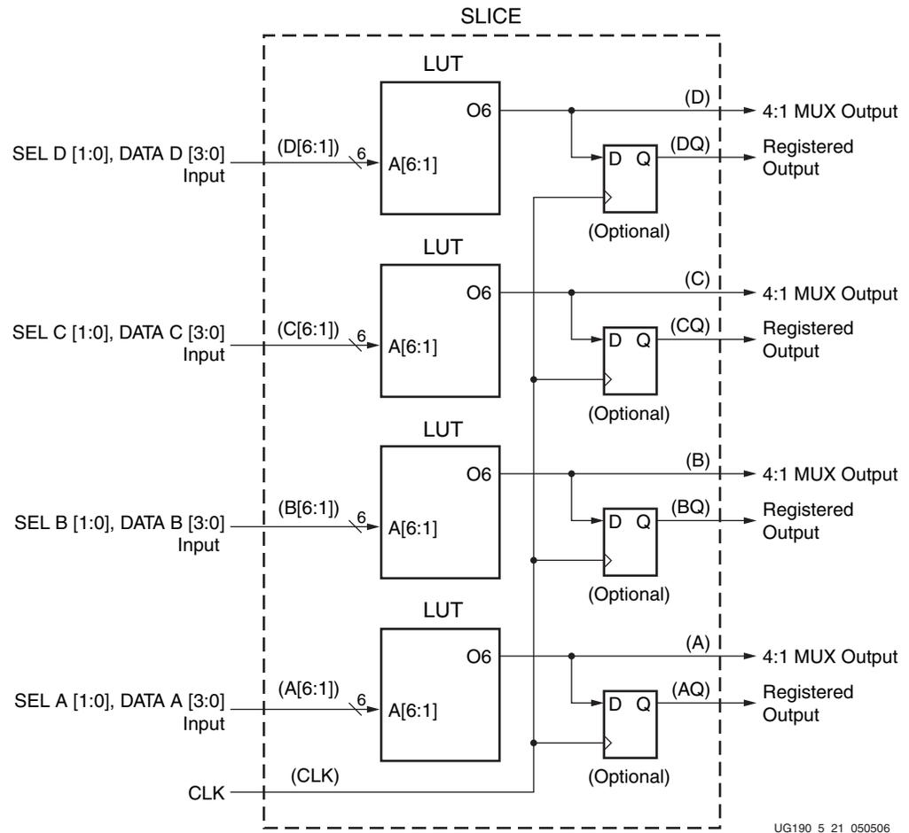
Figure 5-21: Four 4:1 Multiplexers in a Slice
