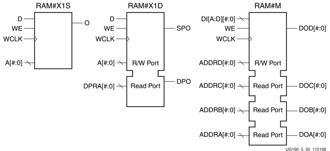
Figure 5-32: **Single-Port, Dual-Port, and Quad-Port Distributed RAM Primitives**
