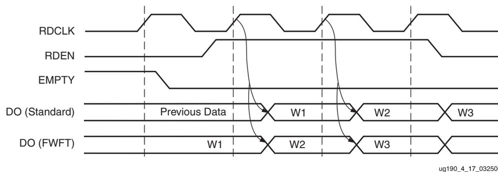
Figure 4-20: Read Cycle Timing (Standard and FWFT Modes)
