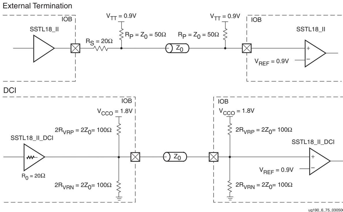
Figure 6-80: SSTA18 (1.8V) Class II Unidirectional Termination
