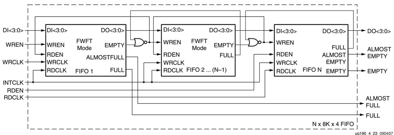
Figure 4-26: Example: Cascading Multiple FIFOs by Depth
