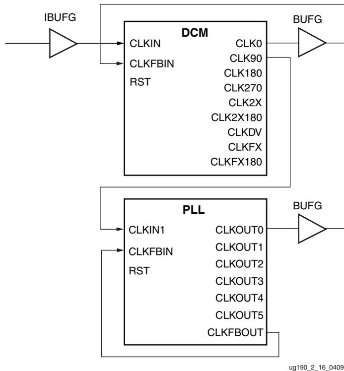
Figure 2-15: Direct Connection between DCM and PLL
