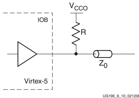
Figure 6-12: Driver with Termination to  $V_{CC0}$  without DCI
