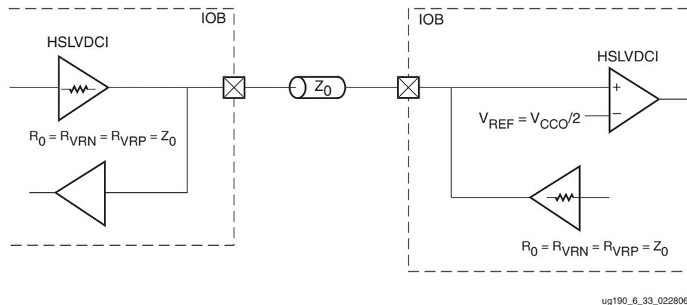
Figure 6-35: HSLVDCI Controlled Impedance Driver with Bidirectional Termination
