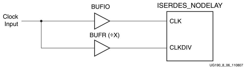
Figure 8-6: Clocking Arrangement Using BUFIO and BUFR
