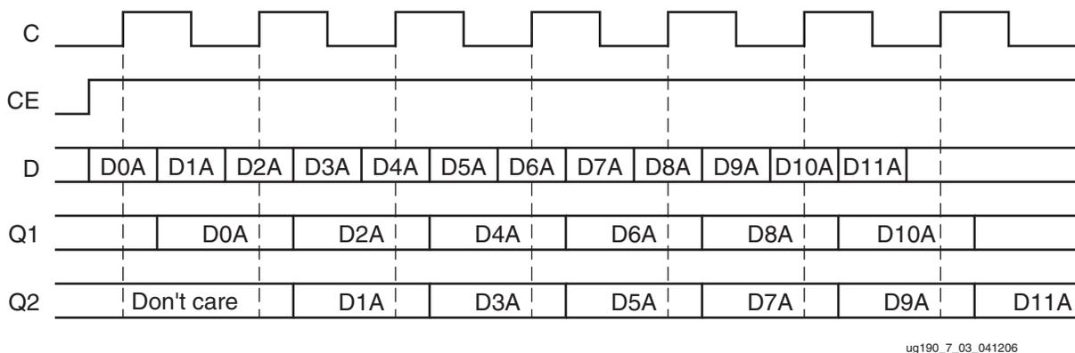
Figure 7-3: Input DDR Timing in SAME\_EDGE Mode
