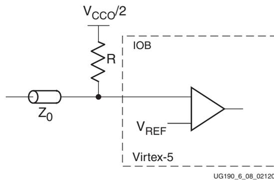
Figure 6-10: Input Termination to  $V_{CCO}/2$  without DCI
