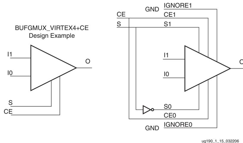
Figure 1-15: BUFGMUX\_VIRTEX4 with a CE and BUFGCTRL
