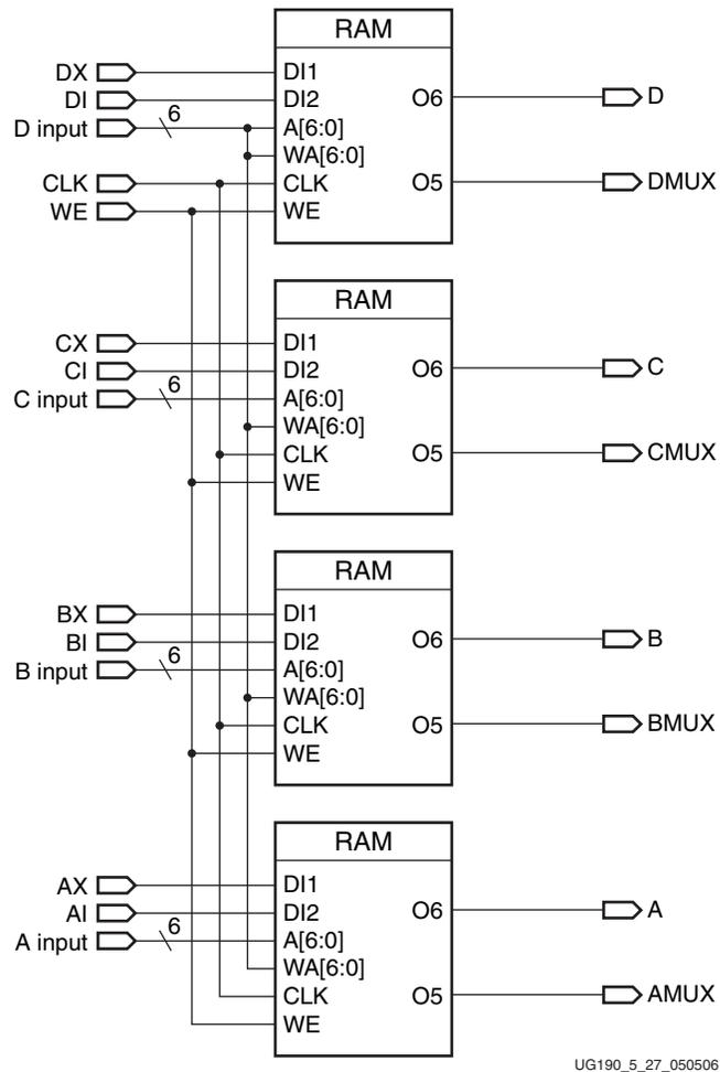
Figure 5-27: Simplified Virtex-5 FPGA SLICEM Distributed RAM
