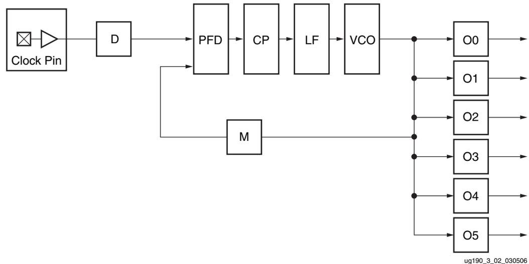
Figure 3-2: Block Diagram of the Virtex-5 FPGA PLL
