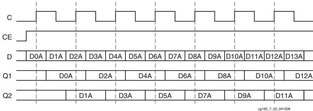
Figure 7-2: Input DDR Timing in OPPOSITE\_EDGE Mode
