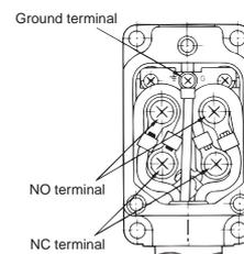
**Note:** The ground terminal is only installed on models with ground terminals.
