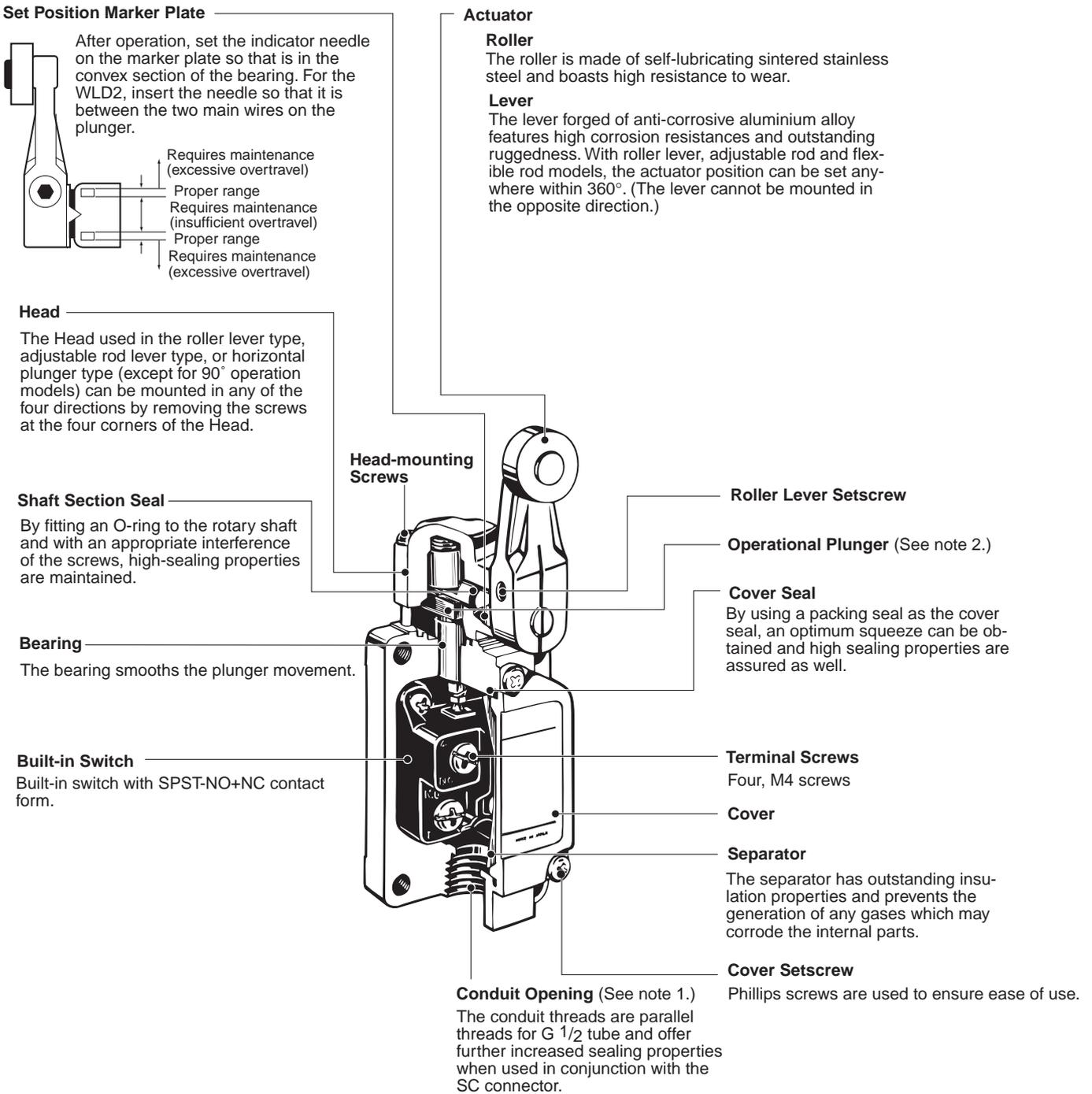
**Note 1.** The display for conduit threads has changed from PF<sup>1</sup>/<sub>2</sub> to G<sup>1</sup>/<sub>2</sub>, according to revisions of JIS B 0202. This is only a change in the display, so the thread size and pitch have not changed. (Conduit threads Pg 13.5 and <sup>1</sup>/<sub>2</sub>-14NPT are also available.)
