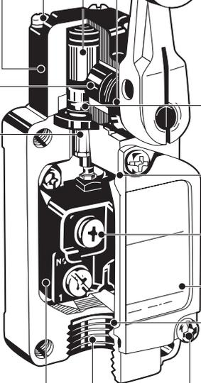
\* By changing the direction of the operational plunger, any one of the three operational directions (both sides, left, or right) can be selected.
