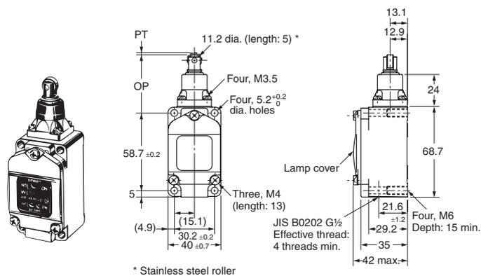
**Sealed Top-roller Plunger (Pre-wired connectors)**
