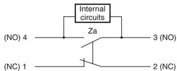
**Direct-wired Connector, Pre-wired Connector, and Indicator-equipped (Light-ON when Not Operating) Switches \*1**
