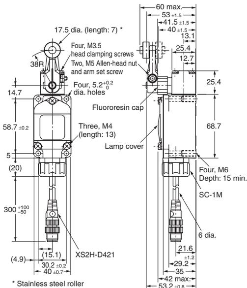
**Sealed Top-roller Plunger (Screw Terminals)**
