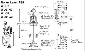
Note: 1. WL□G2 is identical to other models except in the shape of the set position marker plate.
