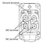
The ground terminal is only installed on models with ground terminals.
