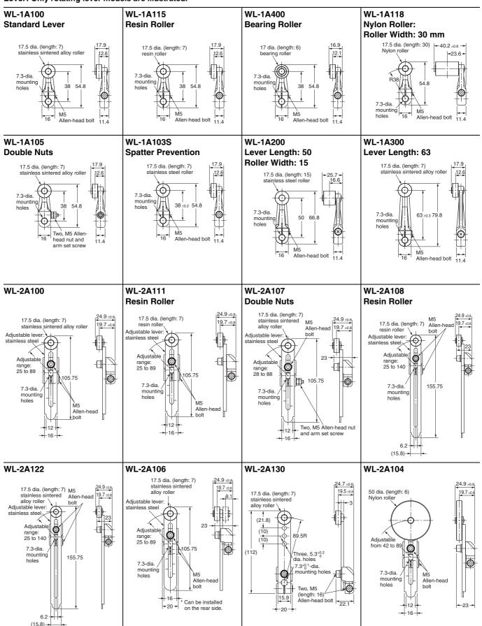
Note: Unless otherwise indicated, a tolerance of  $\pm 0.4$  mm applies to all dimensions.
