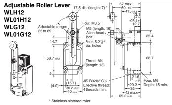
Note: 1. WL G12 is identical to other models except in the shape of the set position marker plate. 2. The built-in switch for WLH12 is W-10FB3.
