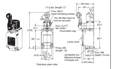
Roller Lever (Pre-wired connectors) WLCA2-□S-M1J\*/WL01□-□S-M1J\* WLH2-□S-M1J\*/WLG2-□S-M1J\*
