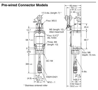
Note: 1. Only the dimension of the set position marker plate is different for WLG2 Models.
