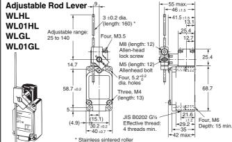
Note: 1. WL $\square$ GL is identical to other models except in the shape of the set position marker plate.
