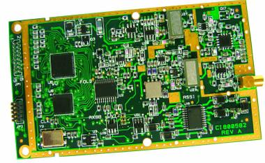
**Powerful.** With a full 1/2 watt transmit power and a receive sensitivity of -103dBm, the WIT910 can achieve ranges in excess of 20 miles using 3dB omni-directional antennas. When long range isn't needed, the WIT910, measuring just 80.2mm x 46.5mm x 8.6mm and weighing just 35 grams, is a powerful performer at low power, consuming less than 100mA at 3.3 volts.
