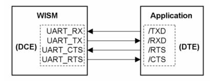
Port UART\_TX transmits data to the application's /RXD input.
