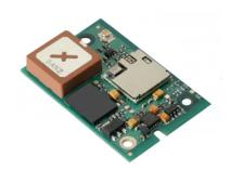
They are ideal for low power M2M applications where cable replacement is the primary requirement. They also feature PCM support for voice applications, including eSCO operation. The BISM2 PA module is the industry's most efficient long range Bluetooth module, with open field ranges in excess of 1km.
