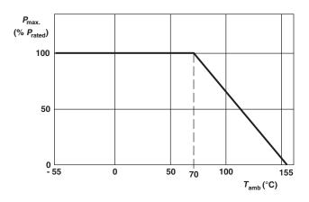
Maximum dissipation ( $P_{\text{max}}$ ) in percentage of rated power as a function of the ambient temperature ( $T_{\text{amb}}$ )
