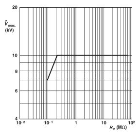
Maximum allowed peak pulse voltage in accordance with "IEC 60065 chapter 14.1"; 50 discharges from a 1 nF capacitor charged to  $\hat{V}_{\text{max}}$ ; 12 discharges/minute (drift  $\Delta R/R \leq 2$  %)
