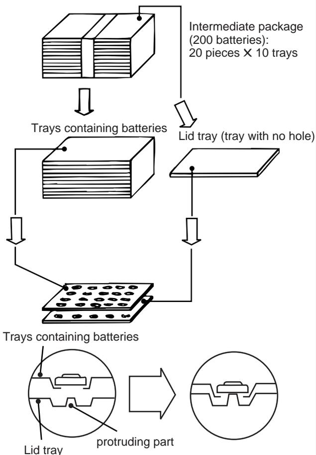
\*Lay a tray lid flat and place a tray containing batteries on top of it: batteries are pushed up by protrusions of the lid tray so that they can be easily picked up with fingers.
