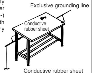
Battery-mounted PC boards were inadvertently brought into contact with spacers and a conductive rubber sheet. The battery charge was exhausted.
