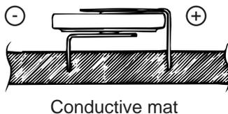
A battery was placed directly on a rubber sheet spread over a worktable. The (+) and (-) terminals were in contact with the sheet and the battery charge was exhausted.
