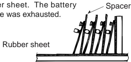
When batteries are to be used near protective materials, take every possible care to ensure that the (+) and (-) terminals of the batteries or PC boards, etc. on which batteries are mounted do not touch these protective materials directly.
