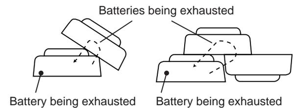
\*Contact of batteries with each other forms discharge circuits, thus the batteries are drained.
