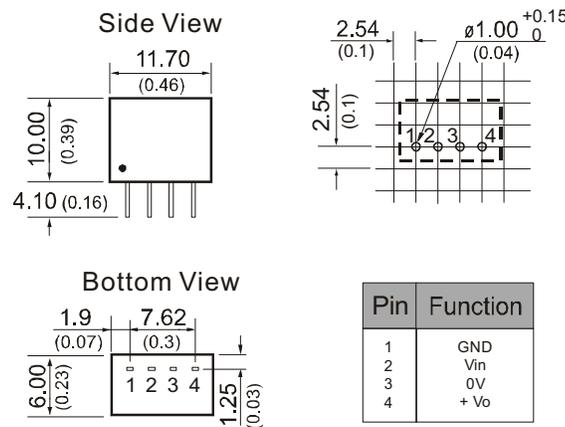
Note: All Pins on a 2.54mm(0.1) pitch; All Pin diameters are 0.50 mm(0.02); Tolerances: ±0.25mm(0.01); Unit: mm(inch).
