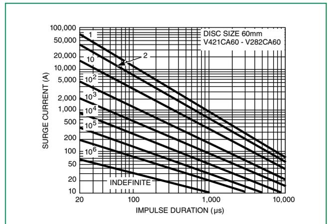
NOTE: If pulse ratings are exceeded, a shift of  $V_{NDCI}$  (at specified current) of more than  $\pm 10\%$  could result. This type of shift, which normally results in a decrease of  $V_{NDCI}$ , may result in the device not meeting the original published specifications, but does not prevent the device from continuing to function, and to provide ample protection.
