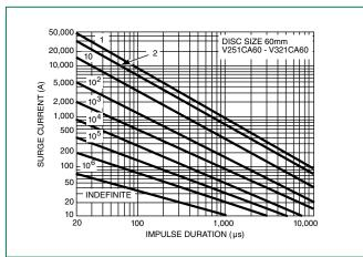
NOTE: If pulse ratings are exceeded, a shift of  $V_{\text{NDCI}}$  (at specified current) of more than  $\pm 10\%$  could result. This type of shift, which normally results in a decrease of  $V_{\text{NDCI}}$  may result in the device not meeting the original published specifications, but does not prevent the device from continuing to function, and to provide ample protection.
