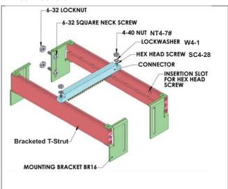
To mount connectors, simply slide nut into desired position and fasten with screws and lockwasher as illustrated. SC4-28 screws available in bulk quantities.
