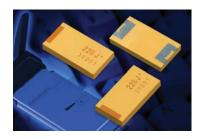
TLN PulseCap™ Tantalum Capacitors offer low profile and high capacitance solution for applications where boosting power is required together with need for reduced height. Typical applications are PCMCIA/USB wireless express cards where bulk capacitance is needed to boost transmitter power. PulseCap™ provides high capacitance 2200µF in a maximum height of 2.0 mm and voltage rating 6.3V.
