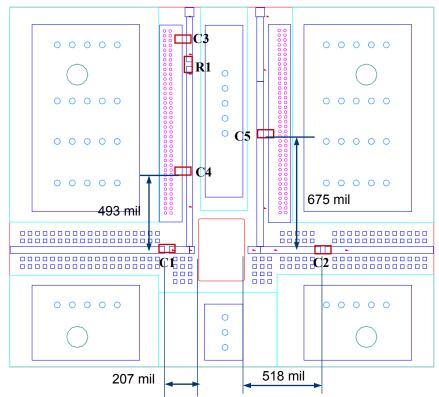
\*The layout is a general purpose drawing that needs to be tuned for the specific application. PCB is RO4003 20 mil thickness, 0.5 oz standard copper cladding, with  $\varepsilon_r$  = 3.38.
