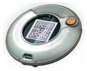
graphical user interface and game demos. Includes evaluation board (USB, LCD), integrated debugging/ programming via USB (RLink), software toolset (RIDE - debug code up to 32 K, GNU C /C++ compiler) and application sources. ST order code: STM3210B-PRIMER
