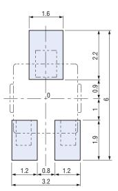
Note) The zero point is the center of mounting.
