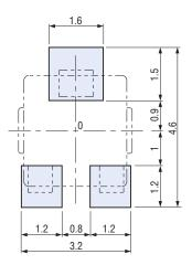
For reflow soldering
