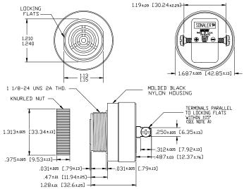
NOTE A: TERMINALS-032 BRASS TIN PLATED, TAPPED FOR #6-32 SCREW. TWO #6-32 NICKEL PLATED BRASS SCREWS INCLUDED. WILL ACCEPT 1/4' QUICK CUNNECT. NOTE B: MOUNTING- REMOVE BLACK PLASTIC NUT AND INSERT THREADED FRONT THROUGH 1.25' HOLE PUNCHED IN PANEL, IF DRIENTATION IS NEEDED, NOTE LOCKING FLATS ON DRAVING, SCREW NUT BACK ON. DO NOT OVERTIGHTEN.
