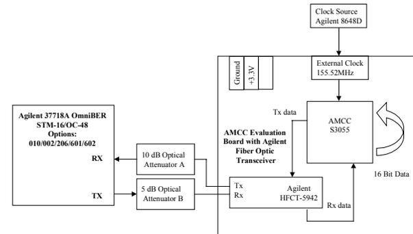
**Figure 6. Block diagram and measurement setup for AMCC S3055 reference design.**
