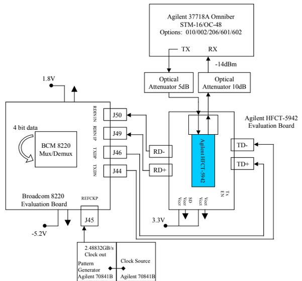
Figure 20. Block diagram of jitter measurement setup between the Agilent HFCT-5942 and the Broadcom BCM8220.
