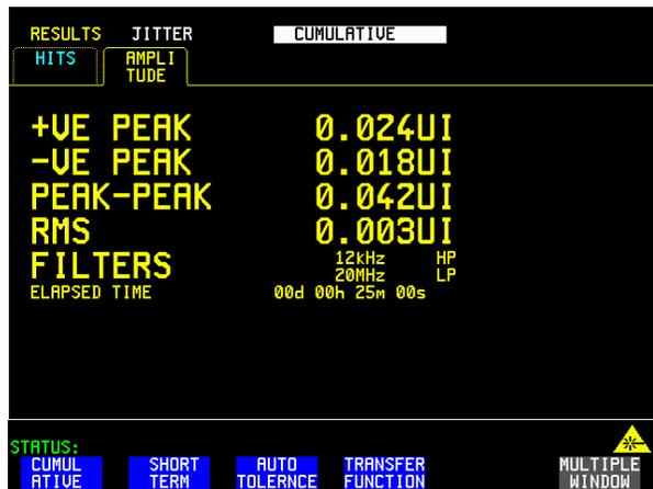
Figure 21. Jitter generation result as measured with the setup described in Figure 20.
