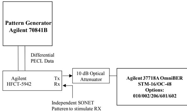
**Figure 5. Measuring jitter generation of HFCT 5942.**
