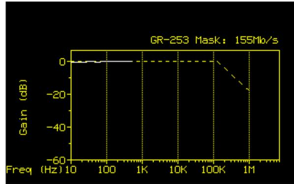
**Figure 14. Low frequency jitter tolerance of Agilent/Vitesse reference board at OC-3.**
