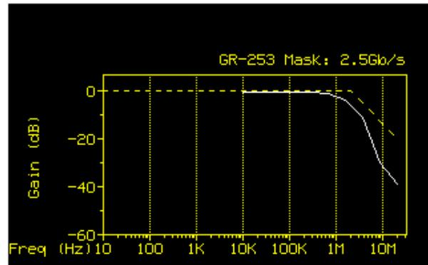
Figure 19. High frequency jitter transfer of Agilent/Vitesse reference board at OC-48.
