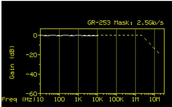
Figure 16. Low frequency jitter transfer of Agilent/Vitesse reference board at OC-48.
