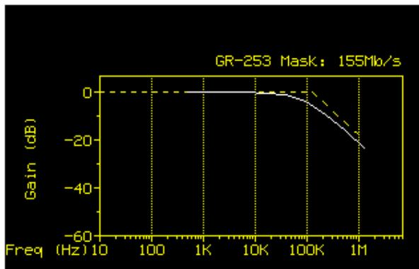
Figure 17. High frequency jitter transfer of Agilent/Vitesse reference board at OC-3.
