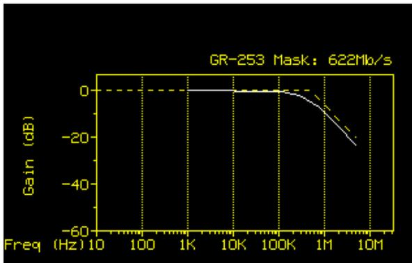
Figure 18. High frequency jitter transfer of Agilent/Vitesse reference board at OC-12.
