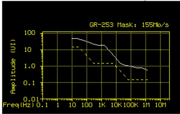
**Figure 11. Jitter tolerance of Agilent/Vitesse reference board with GR-253 mask at OC-3**
