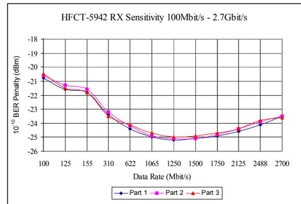
Figure 4. Sensitivity at BER  $10^{-10}$  as a function of data rate.
