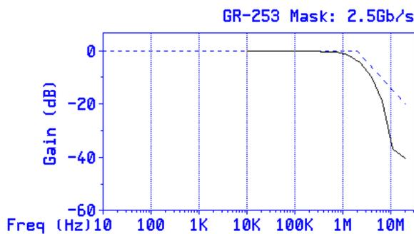
**Figure 9. High frequency jitter transfer of AMCC S3055 and Agilent HFCT-5942**
