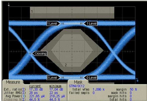
Figure 2. Optical eye of HFCT-5942 at OC-12 using the OC-12 mask and filter.
