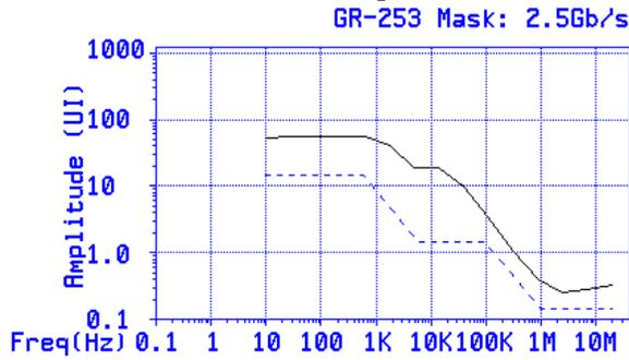
**Figure 7. Jitter tolerance results of AMCC S3055 with Agilent HFCT-5942L.**
