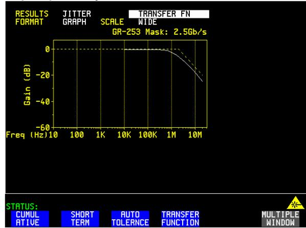
Figure 24. The HFCT-5942 and BCM8220 fulfills the high frequency GR-253 jitter transfer mask.
