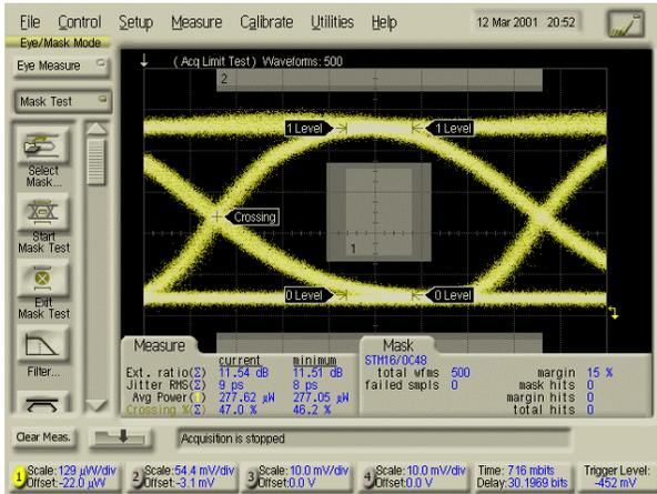
Figure 1. Optical eye using SONET OC-48 optical filter and SONET OC-48 eye mask. Mask margin of 15% and extinction ratio greater than 10dB are typical.
