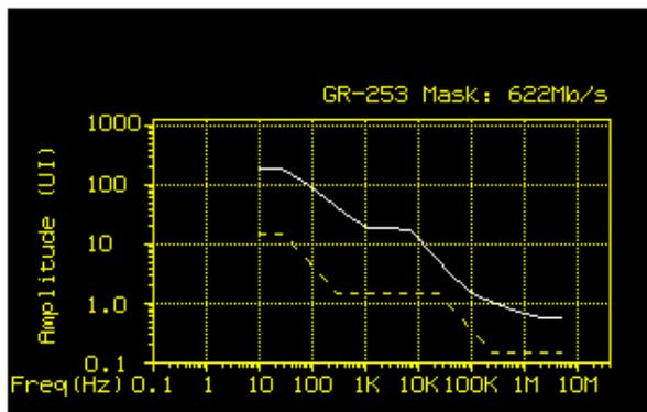
**Figure 12. Jitter tolerance of Agilent/Vitesse reference board with GR-253 mask at OC-12.**
