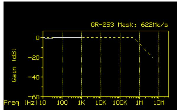
**Figure 15. Low frequency jitter transfer of Agilent/Vitesse reference board at OC-12.**
