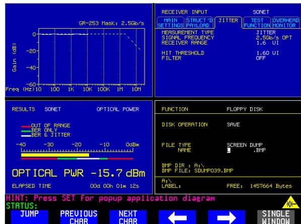
Figure 23. The HFCT-5942 and BCM8220 fulfills the low frequency GR-253 jitter transfer mask.
