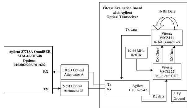
**Figure 10. Block diagram and measurement setup for the Vitesse/Agilent OC-48 reference design.**
