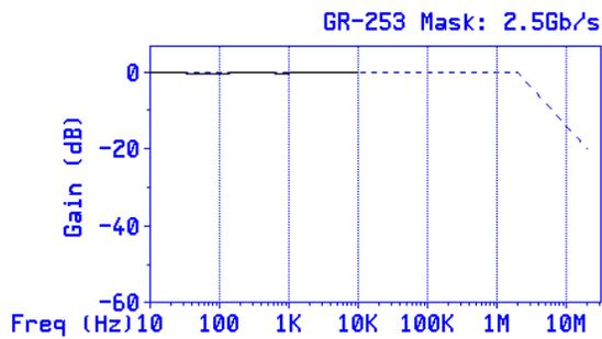
**Figure 8. Low frequency jitter transfer of AMCC S3055 and Agilent HFCT-5942**
