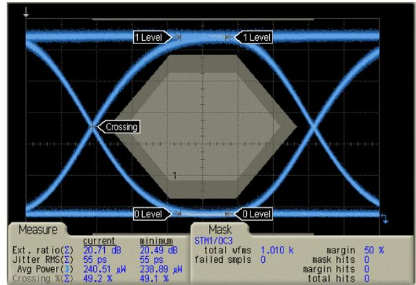
Figure 3. Optical eye of HFCT-5942 at OC-3 using the OC-3 mask and filter.
