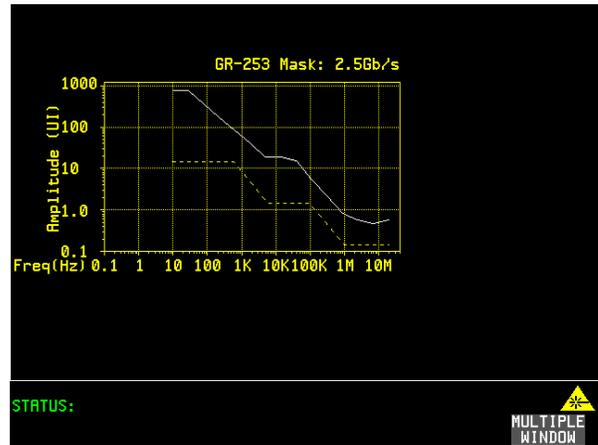
Figure 22. The HFCT-5942 and BCM8220 fulfills the GR-253 jitter tolerance mask.
