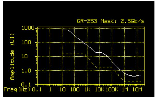
**Figure 13. Jitter tolerance of Agilent/Vitesse reference board with GR-253 mask at OC-48 data rate.**
