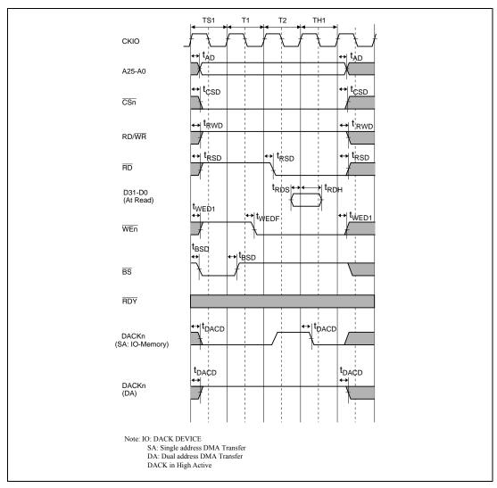
Figure 9.5 Memory Byte control SRAM Bus cycle Basic Read cycle (No wait, Address set up/Insert hold time, AnS=1, AnH=1)
