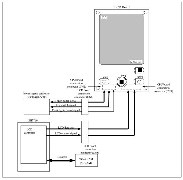
Figure 5.6 LCD Control Block
