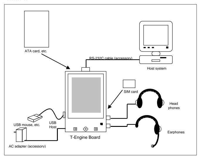
Figure 1.1 System configuration
