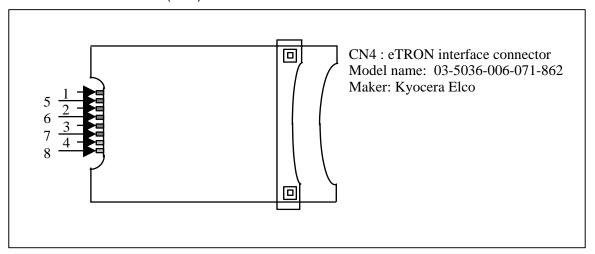
Figure 5.12 eTRON Interface Connector (CN4) Pins
