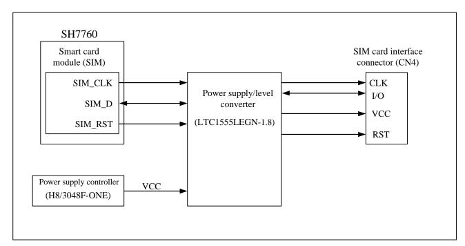
Figure 5.11 eTRON Interface Control Block
