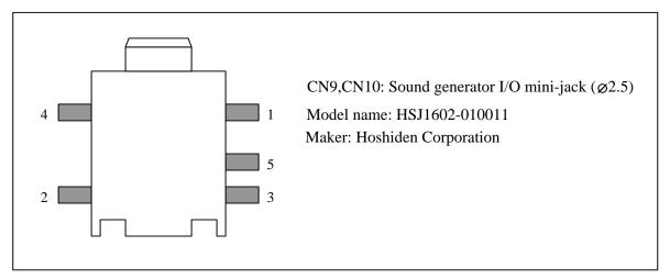
Figure 5.9 Sound Generator I/O Mini-jack (CN9, CN10) Pins
