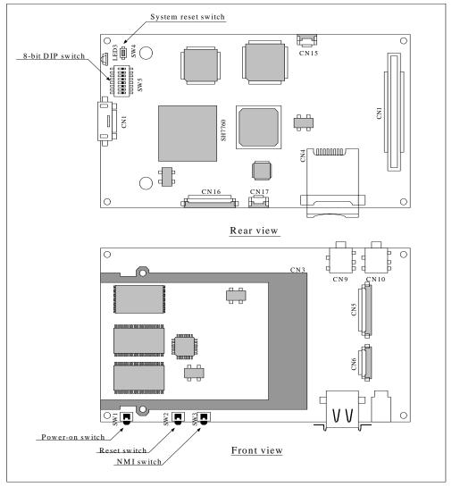
Figure 3.1 CPU Board Switches (SW1 to SW5)
