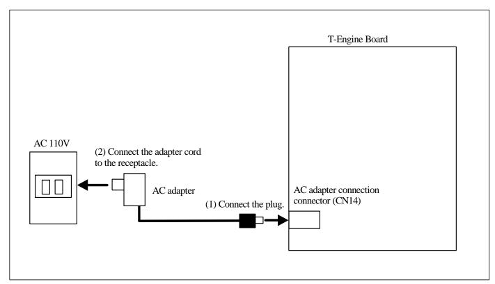
Figure 2.3 AC Adapter Connection Cord
