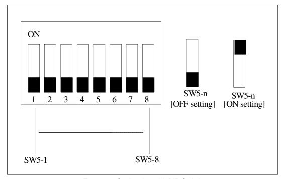
Figure 3.2 Setting the 8-bit DIP Switch
