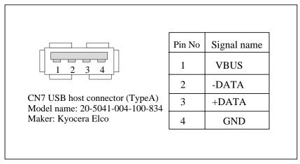
Figure 5.3 USB Host Connector (CN7) Pins
