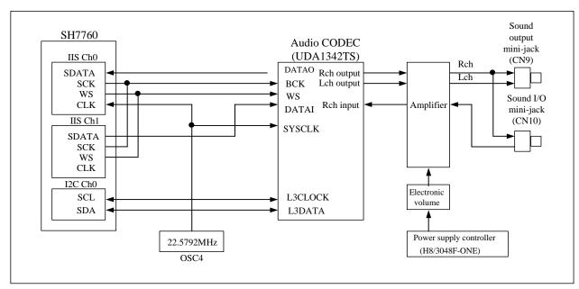
Figure 5.8 Sound Generator Control Block
