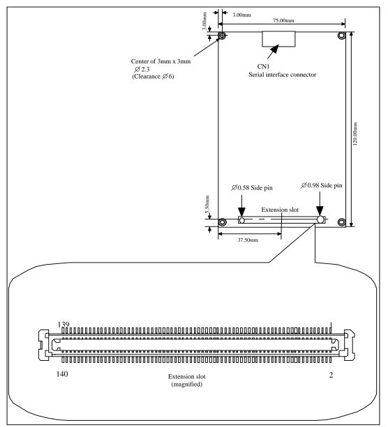
Figure 8.1 Extension Slot Position
