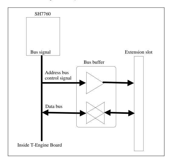
Figure 9.4 Extension Slot Bus Buffer Structure
