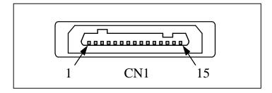
Figure 2.2 Serial Interface Connector Pins
