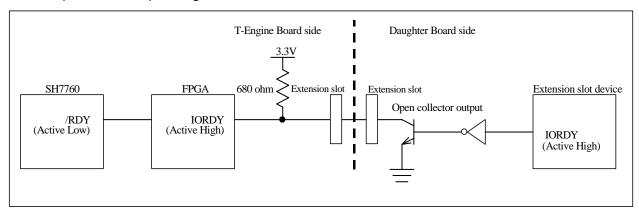
Figure 9.3 Extension Slot IORDY Pin Structure
