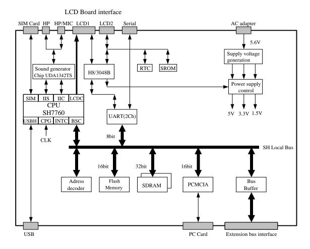
Figure 1.2 T-Engine Block Diagram
