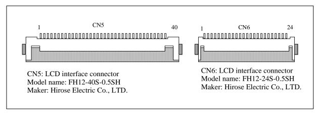
Figure 5.7 LCD Interface Connector (CN5/CN6) Pins
