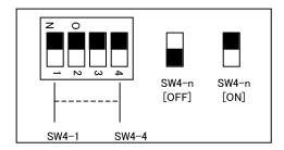
Figure 3.3 Setting the 4-bit DIP Switch
