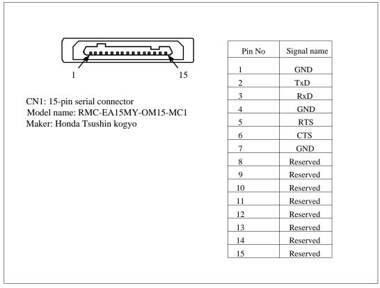
Figure 5.5 15-pin Serial Interface Connector Pins (CN1)
