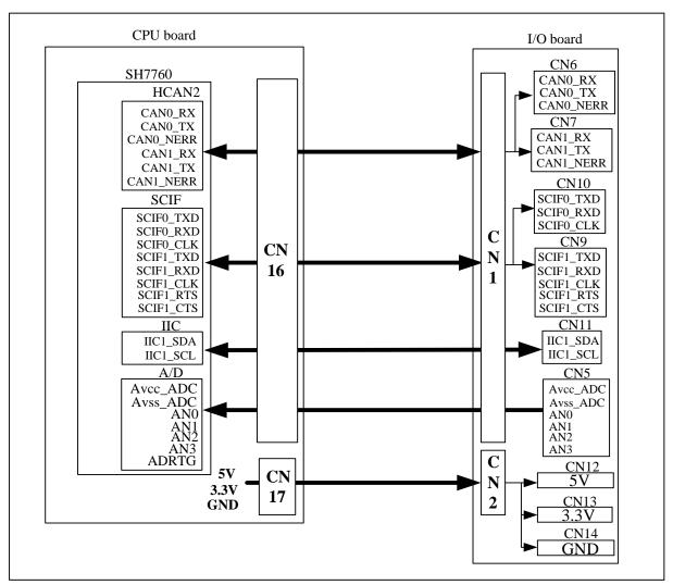
Figure 5.13 I/O Board Control Block
