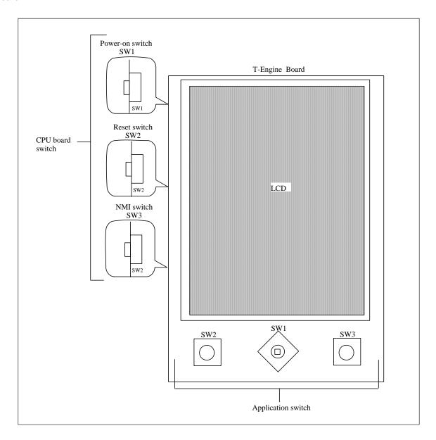
Figure 6.12 T-Engine Switch
