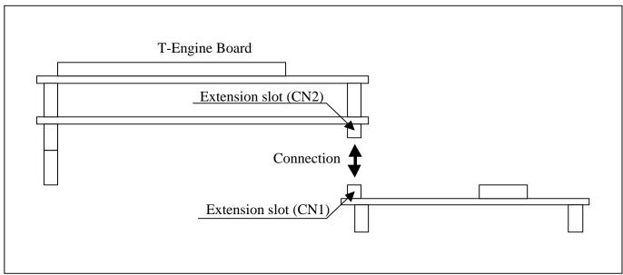
Figure 2.4 Debug Board Connection
