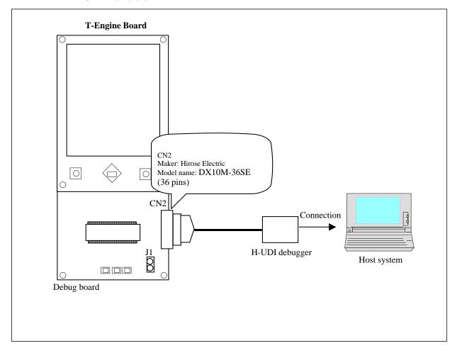
Figure 2.6 H-UDI Debugger Connection
