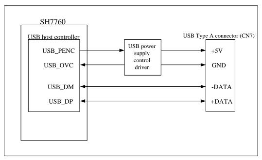
Figure 5.2 USB Host Control Block
