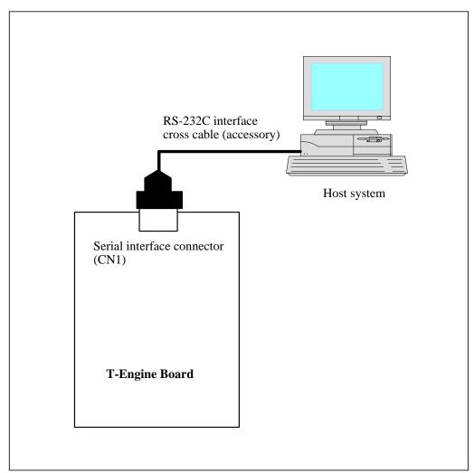
Figure 2.1 Host System Connection
