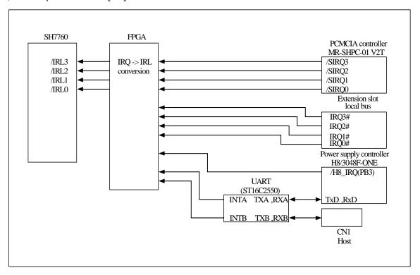
Figure 7.1 Interrupt Signal Mechanism
