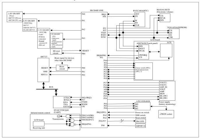
Figure 6.1 Power Supply Control Block Diagram
