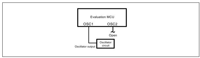
Figure 2.18 External oscillator circuit
