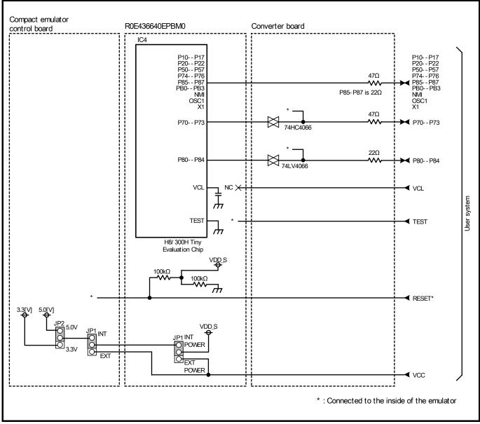
Figure 4.3 Connection diagrams of R0E436640CPE00 (H8/36014, etc.)
