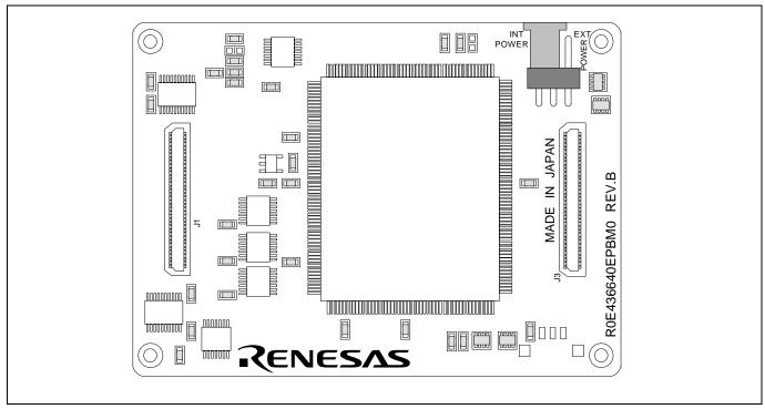
Figure 2.14 Jumper switches on the R0E436640EPBM0
