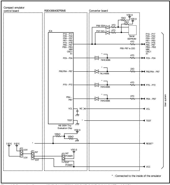
Figure 4.2 Connection diagrams of R0E436640CPE00 (H8/3687, 36087, 36064, 36077 and 36079 etc.)
