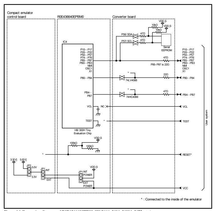
Figure 4.1 Connection diagrams of R0E436640CPE00 (H8/3664, 3694, 36094, 3672, etc.)
