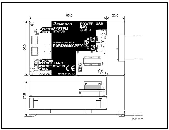
Figure 4.4 External dimensions of the compact emulator
