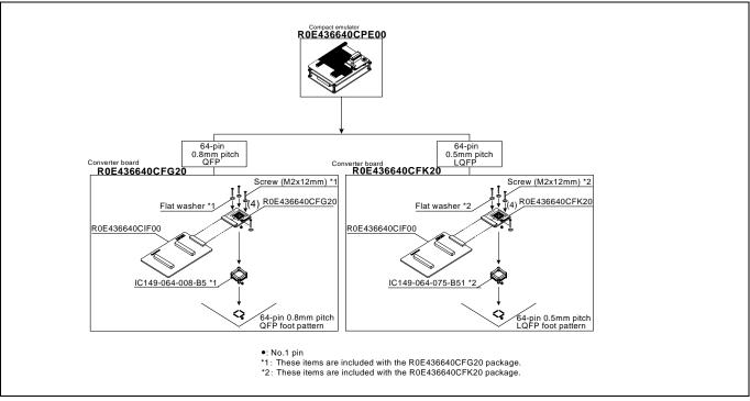
Figure 2.11 Connection of the R0E436640CPE00 and user system
