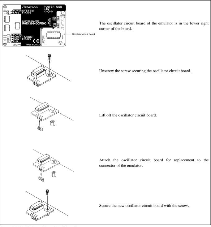
Figure 2.15 Replacing oscillator circuit boards
