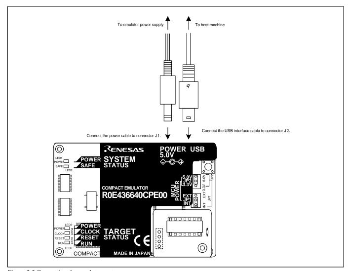
Figure 2.5 Connecting the emulator system
