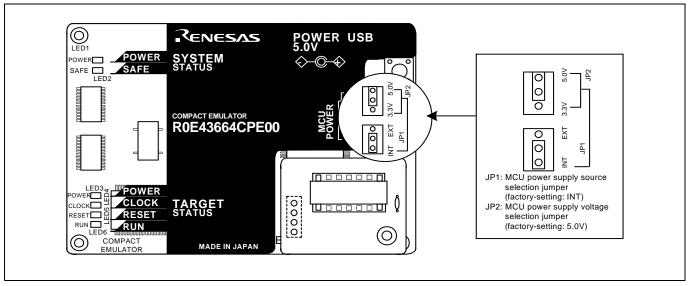
Figure 2.6 Jumper switch locations
