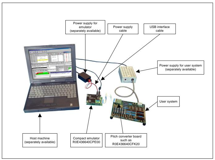
Figure 1.1 System configuration
