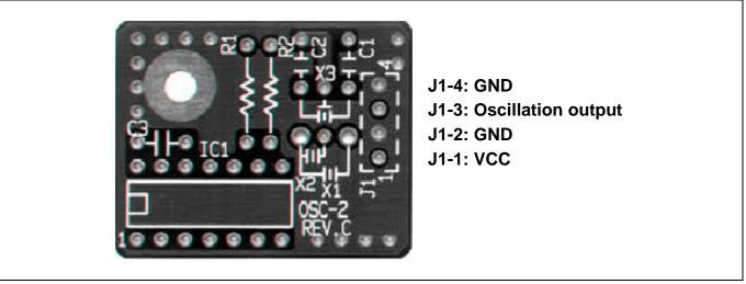
Figure 2.16 External view of the oscillator circuit board OSC-2 and its connector pin locations
