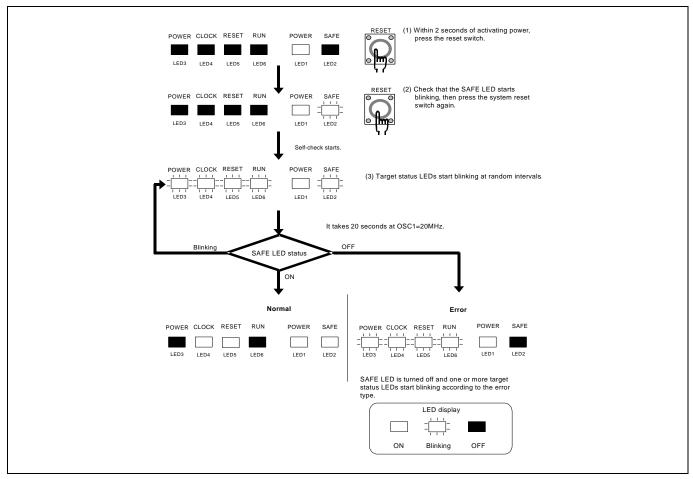
Figure 2.10 Self-check procedure
