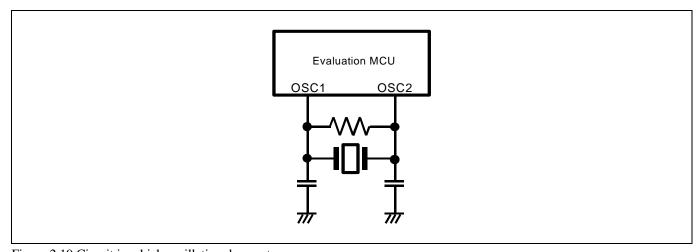
Figure 2.19 Circuit in which oscillation does not occur
