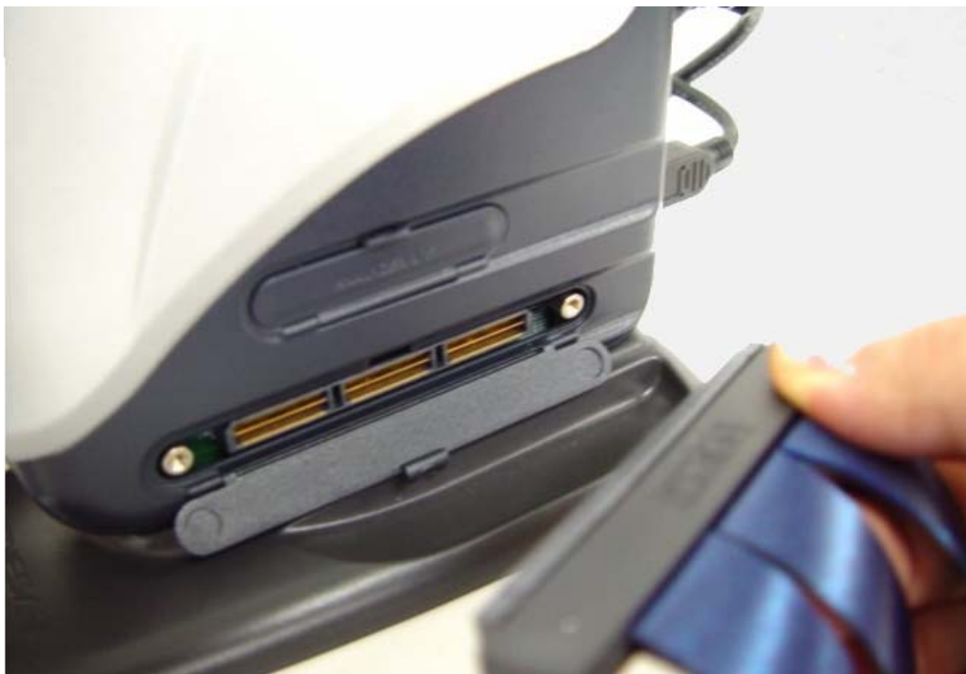
Figure 2.7 Connecting the Trace Cable to E200F
