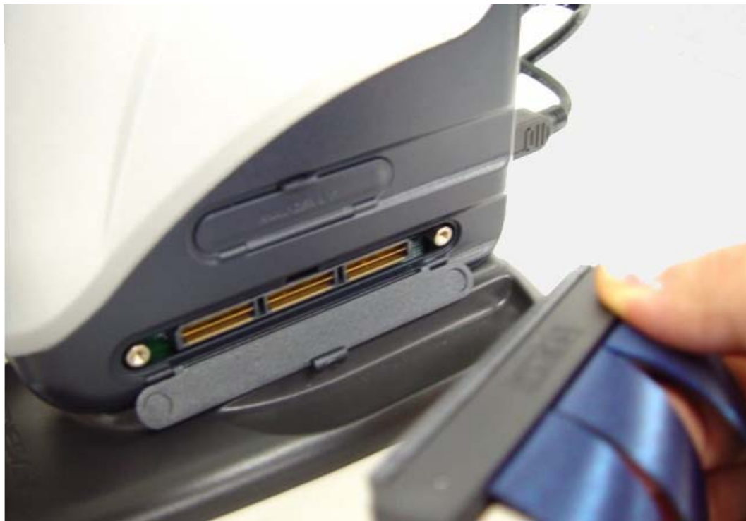
Figure 2.10 Connecting the Trace Cable to E200F
