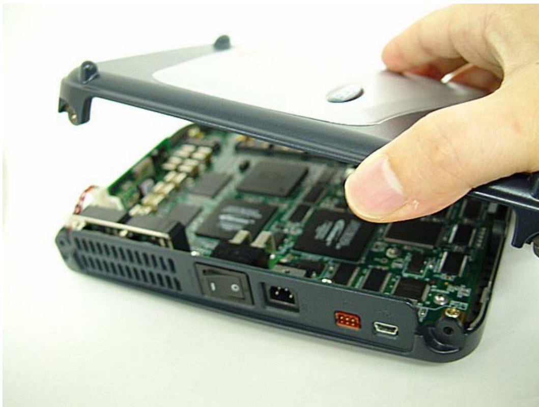
Figure 2.9 Removing the Main Unit Case
