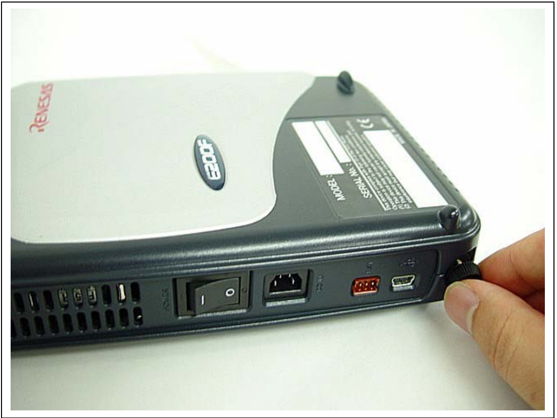
Figure 2.8 Screws for the Main Unit Case
