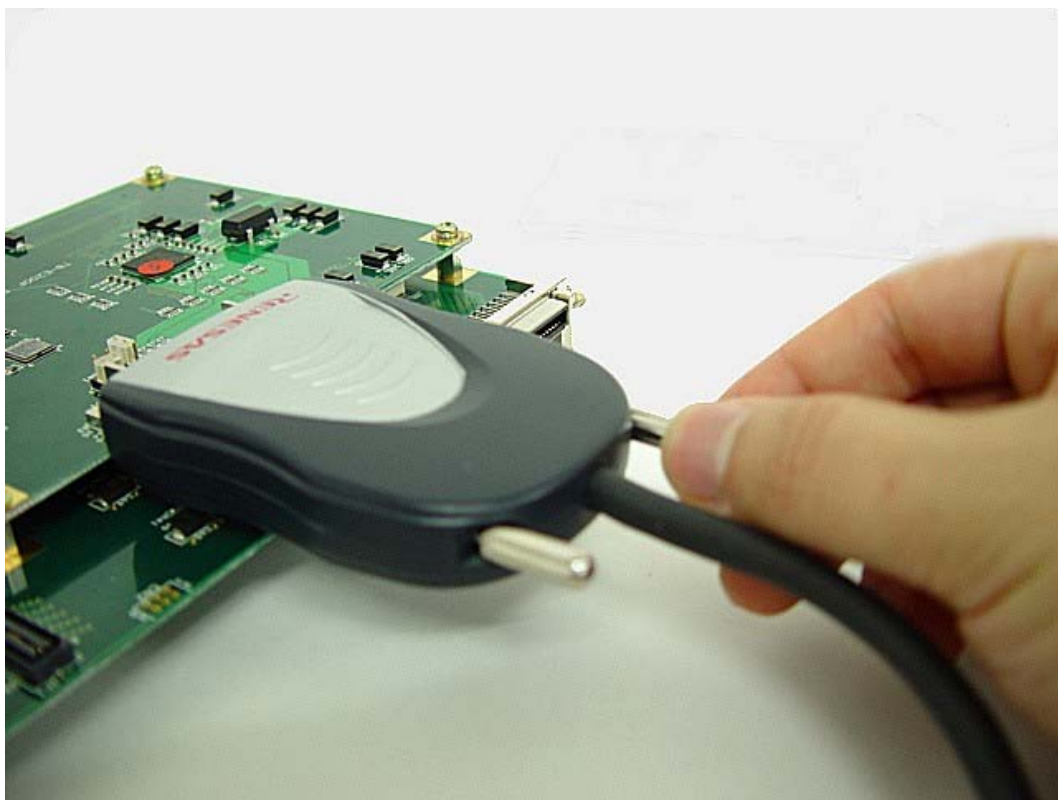
Figure 2.15 Fastening the User System and the H-UDI/AUD Probe
