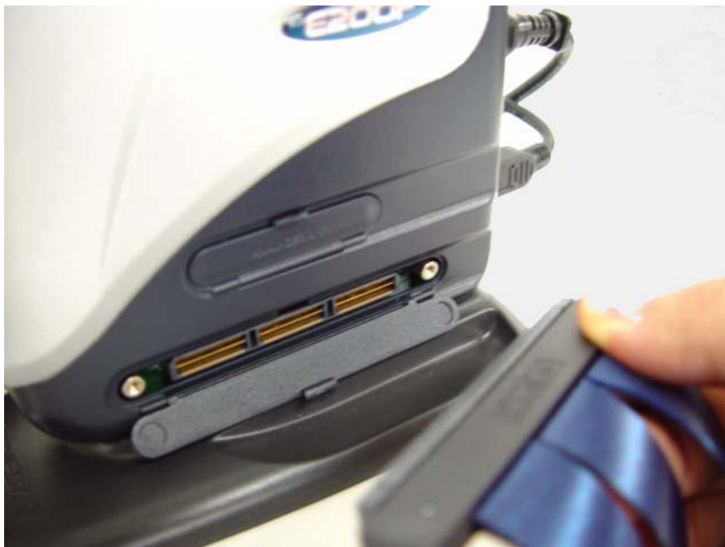
Figure 2.2 Connecting the Trace Cable to E200F
