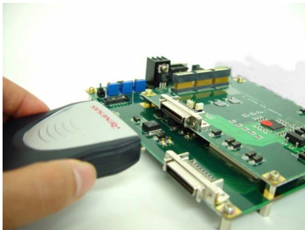
Figure 2.14 Connecting the H-UDI/AUD Probe to the User System
