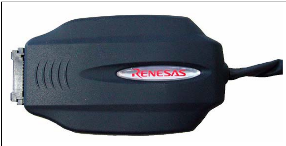
Figure 1.11 38-pin Probe Head Upper View (R0E0200F2EMU00)
