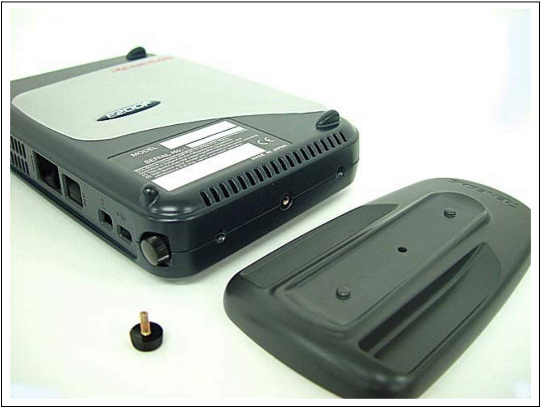
Figure 2.7 Removing the Base Unit for Placing the Emulator Vertically
