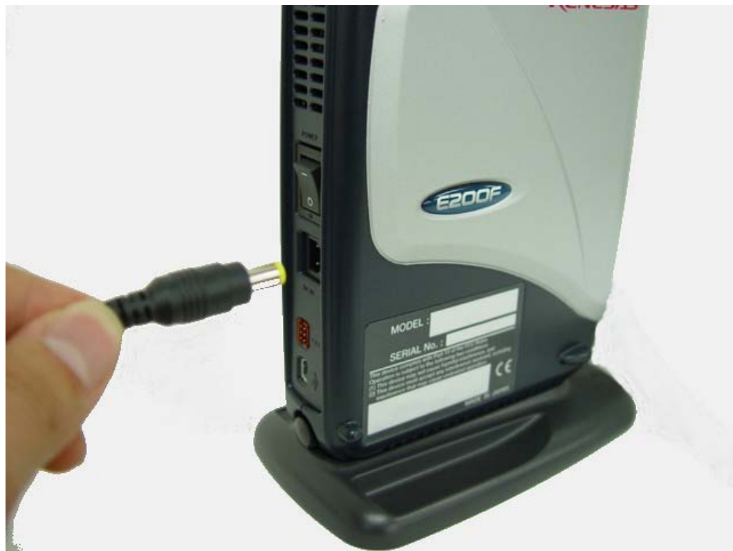
Figure 2.12 Connecting the AC Adapter to the Main Unit Case
