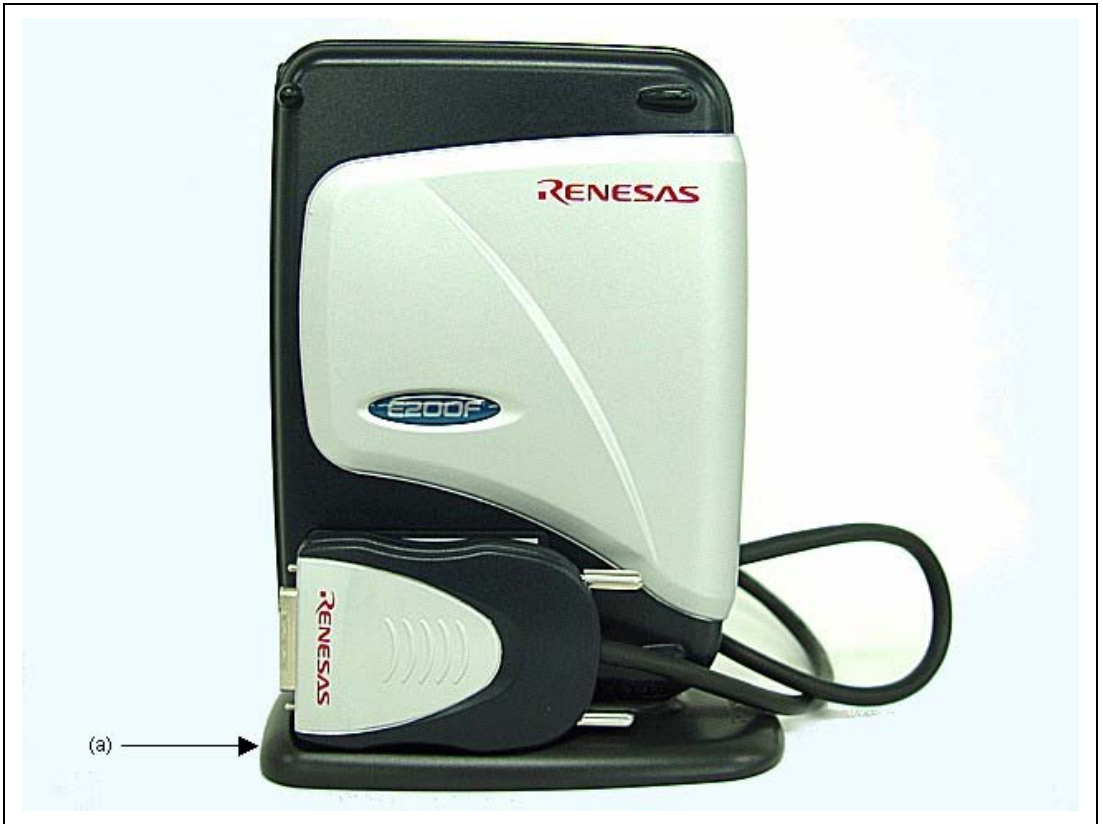
Figure 1.13 Storing the Probe Head (R0E0200F0EMU00)
