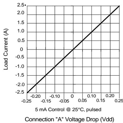
**Figure 3. Linearity Characteristics**
